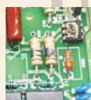
Integrated circuit and resistor damaged by lightning surge
